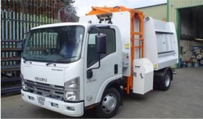
2.2.4 The new fleet will be delivered with new livery to reflect and promote the new services being rolled-out in September-22. All of the large collection vehicles will be fitted with 'electric' bin- lifting equipment which help the vehicles be more fuel efficient and are quieter when working.
