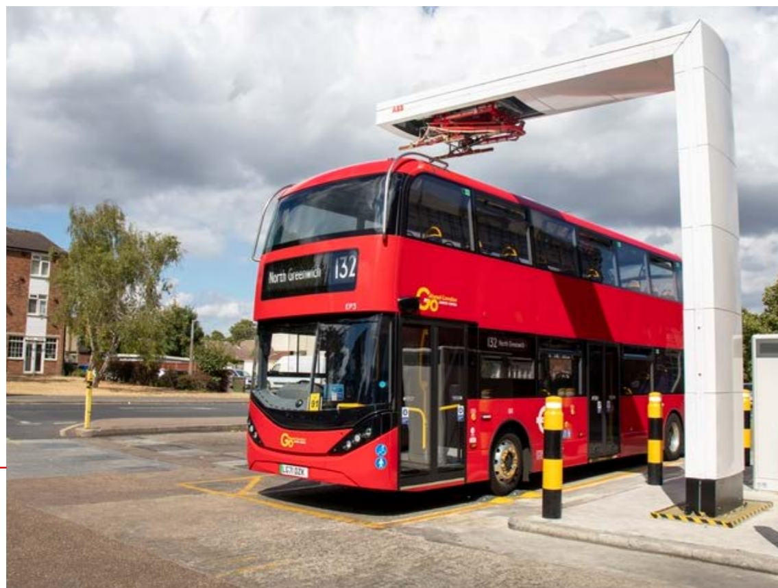
Figure 16. A London bus is charged using a pantograph. (Credit: TfL)
